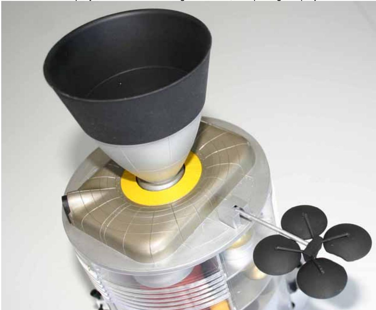
Figure 13 - Main Engine Nozzle
