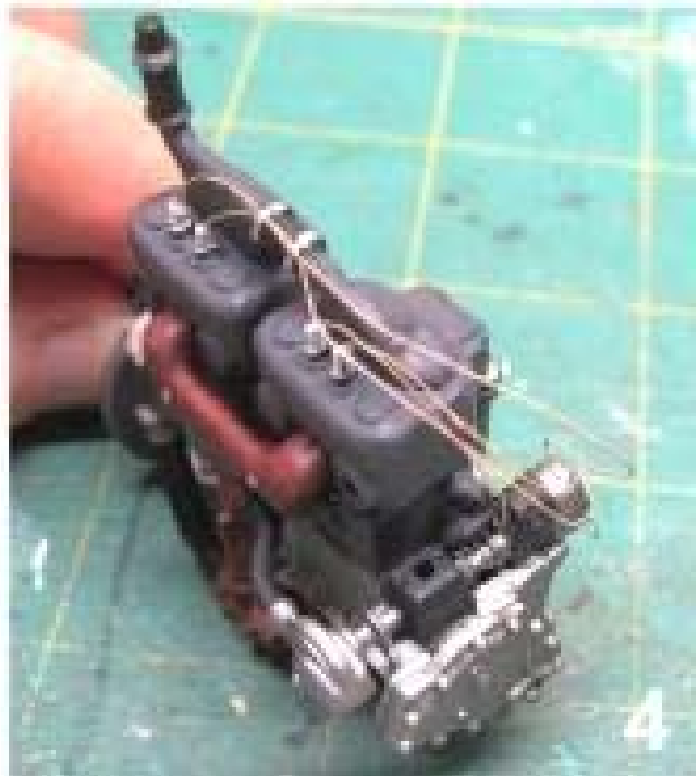
Figure 5 I didn't add a lot of extra detail to this kit, but adding plug wires to the monstrous inline four engine seemed like a requirement. Spark plug detail is already provided. As shown in Figure 5, I first assembled and painted the engine. My first step in wiring the engines was to poke a starter location in the top of each spark plug using a pin. Next, using a #80 drill bit, I drilled out each of the four plugs, as well as four locations on the distributor. My references showed that the distributor is located on part #149 toward the front of the engine. For plug wires, I used 32 gauge wires from the bead aisle of the local hobby store. I glued each end with CA superglue. With the wires in place, I painted them a tan color, simulating fiber insulation.
