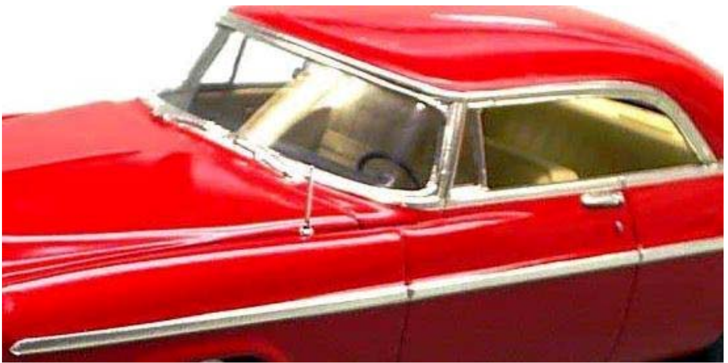
(Fig. #8) After painting, clear-coating, and wet-sanding the body, I applied Bare-Metal foil around the windshield, backlight, side body spears, and front and rear emblems. I was quite dismayed by the fact that all the trim parts to be foiled were not as crisp as I would have expected...even after paint and clear coat. I didn't have that issue with the Hudson Hornet whatsoever.
