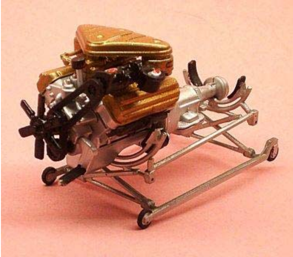
(Fig. #3) I started with the engine, which proved to be a model within itself. The basic components: block/tranny, oil pan, transmission pan, cylinder heads, front cover, and intake manifold should be assembled and painted aluminum. I did so and painted them Testor's Aluminum Plate buffing metalizer.
