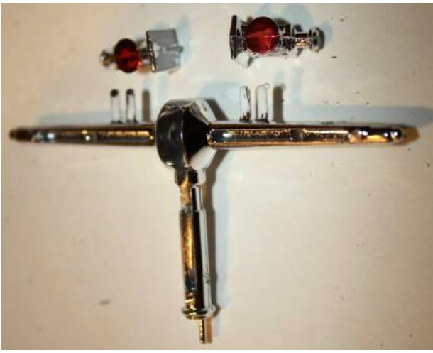
10 The rear end assembly has 3 parts: The main rear end and two tail lights.
