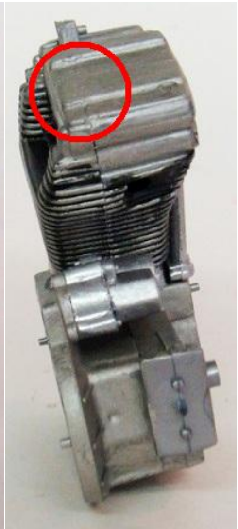
Figure 1708 and Figure 1709 The two engine halves have a seam line that a little Squadron Green Putty will help eliminate.
