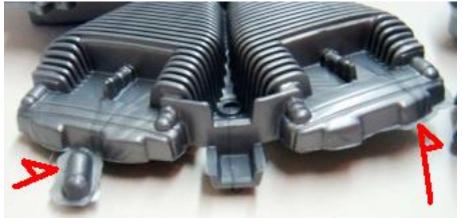
Figure 1705 There is flash on the engine half that will have to be trimmed off.
