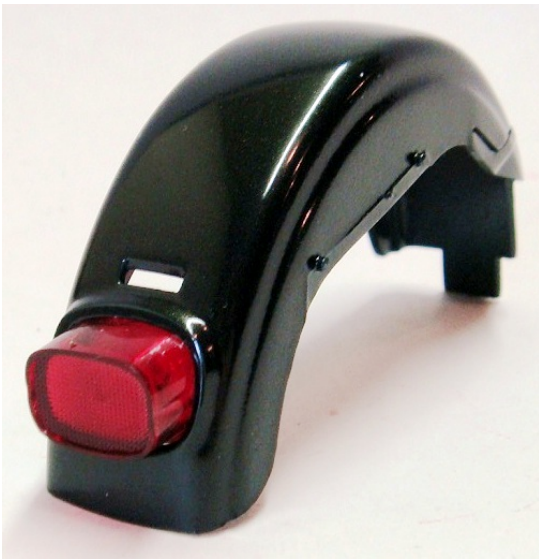
Figure 1704 A view of the completed rear fender after the taillight and rear deflector were installed.
