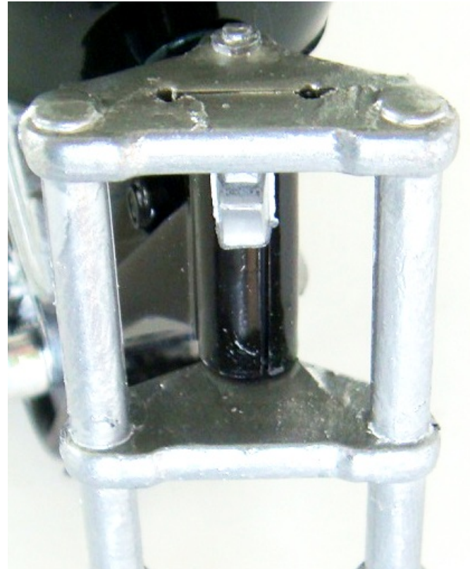
Figure 1718 and Figure 1719 After the Squadron Green Putty is dry I carefully sand it smooth and paint over it with Testors Silver. Now the forks look more realistic like a one piece fork system.
