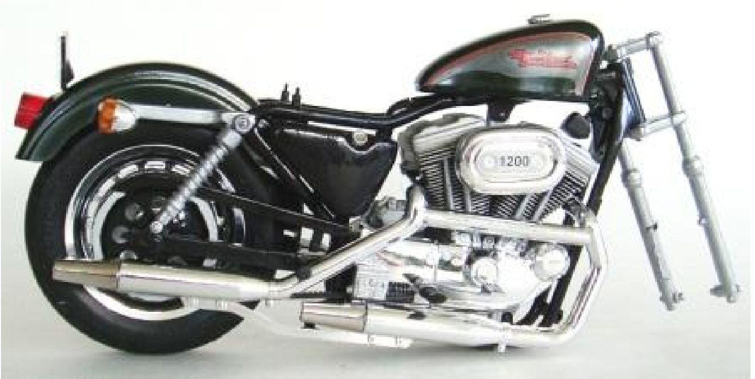
Figure 1723 There are two tail pipes that are glued to the exhaust and then the exhaust system is installed onto the motorcycle assembly.
