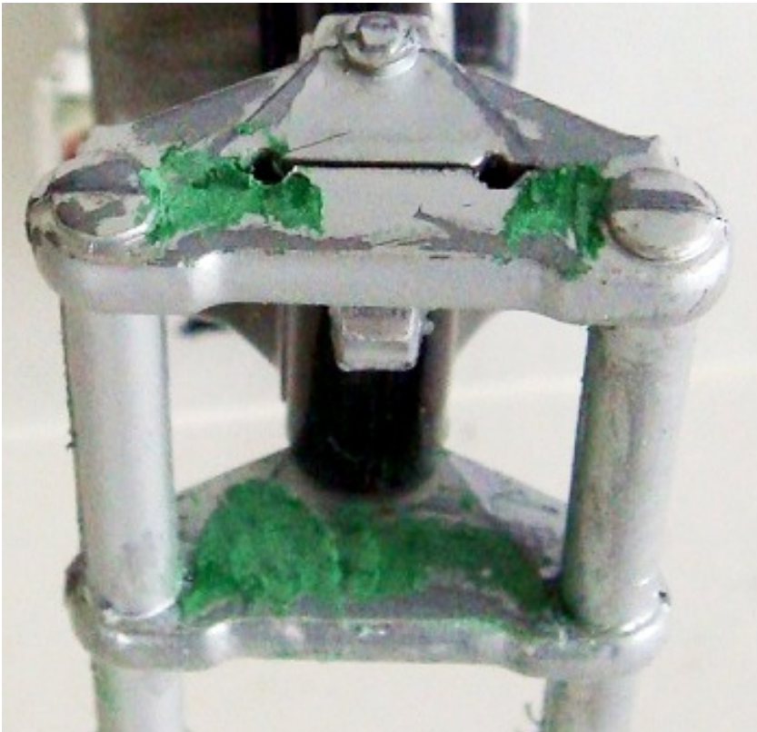
Figure 1718 and Figure 1719 After the Squadron Green Putty is dry I carefully sand it smooth and paint over it with Testors Silver. Now the forks look more realistic like a one piece fork system.
