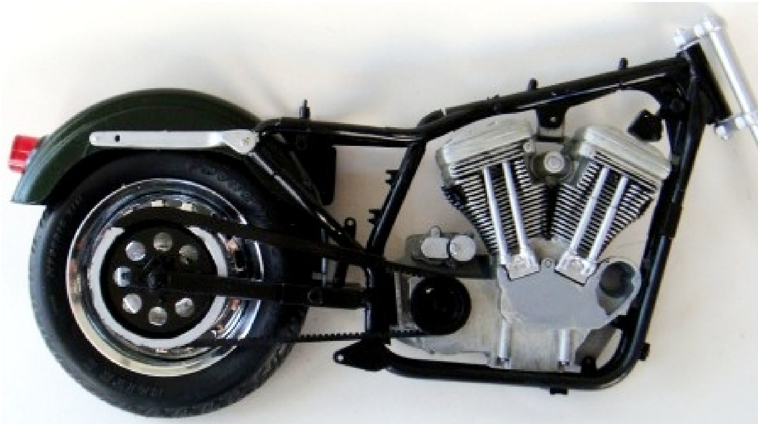
Figure 1713 The rear tire assembly is installed into the motorcycle frame.
