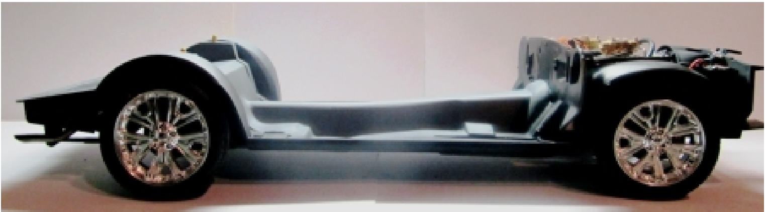
PIC 54 A side shot of the ride height and small rake from the extended shackles.
