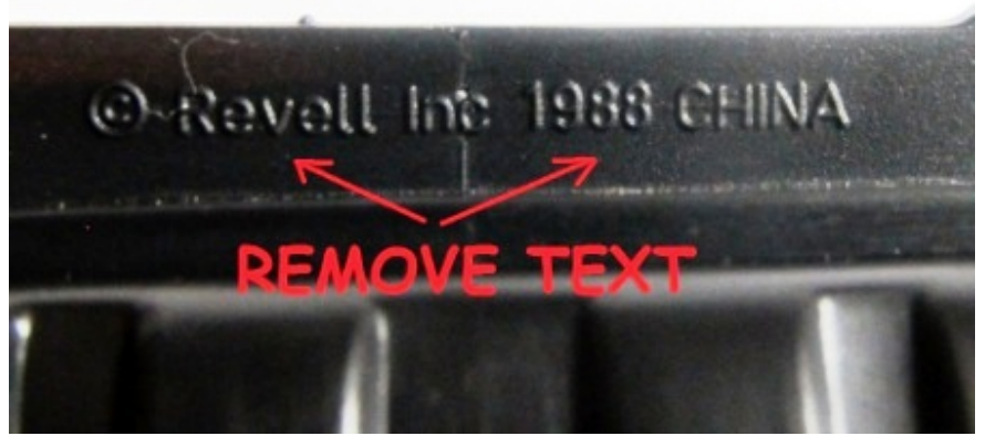
PIC 24 PIC 25 These are the chassis parts to start work on the chassis. As noted in the pic the Copyright text needs to be removed. Scrape it off with a razor blade and sand the area smooth.
