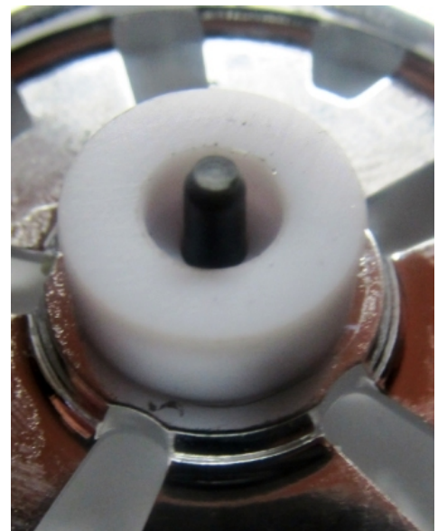
PIC 48 PIC 49 These are the parts to assemble the Foosse wheels. To assemble the pin and retainer on the rim insert the pin into the retainer back and
