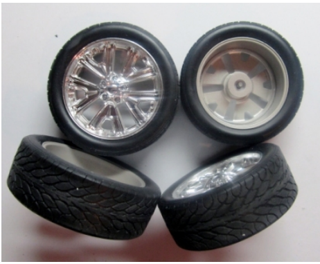
PIC 50 The completed wheels and tires. Assemble by inserting the completed rim into the tire and line up the tire bead to the rim lip. Remember the direction and size differences.
