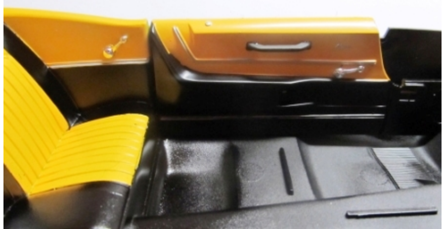
PIC 58 PIC 59 The interior tub and door panels will be first. As I am doing a custom paint on the car the monotone stock look will be replaced with a custom tutone interior. I will use the base body color to highlight the Black interior. The seats will have the fabric center area as a matching color also. The pedals will be painted Flat Black with Silver detail. Primer all the parts you plan to paint. Paint the lightest color or the detail color first. Tape off the area you want to protect the color on and paint the overall color. Assembly: Attach the grab handle and window crank to each door panel. Attach a window crank to each rear panel. Paint the door lock knob and the trim strip Silver. Install Decal #11 on each door panel. The pedals will be installed after the floor is flocked.
