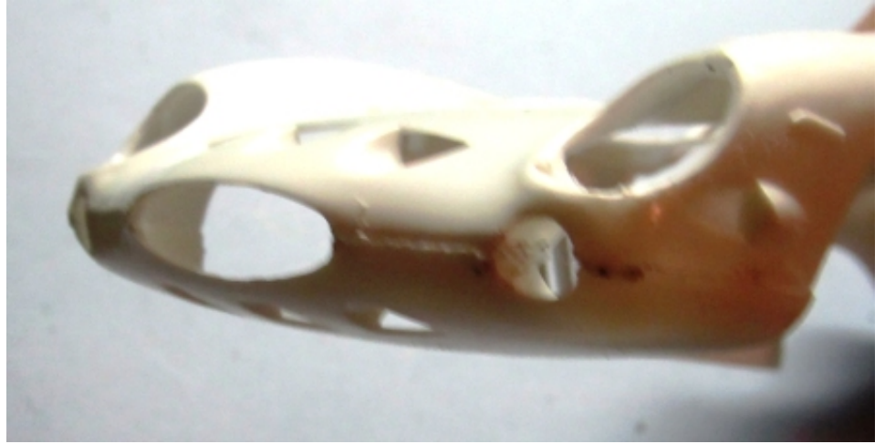
PIC 48 PIC 49 Install all the hinges on the doors, trunk and hood. Install the front pan on the body now.
