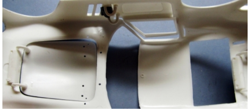
PIC 50 PIC 51 Sand and clean up the lines and prepare the car for Primer. Prior to paint work I went ahead and installed all the panels. I will paint the car as a whole so all the panels will match.
