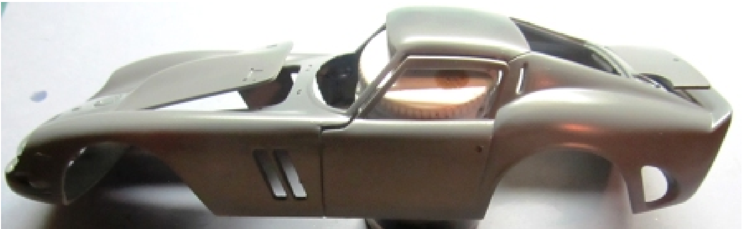
PIC 52 With the car in Primer any further blemishes will show up and can be repaired before you do a final color coat. Check the body over closely, fix any issues and re-prime if necessary. Once the body is correct wet sand the whole thing with 800 grit paper and paint the color coat.
