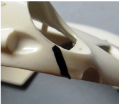
PIC 44 PIC 45 The front fenders have a mold line that runs under the lights across the top of the fender.
