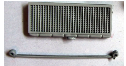
PIC 12 Paint the track bar Black and install it on the pins of the spindles. DO NOT GLUE IT.
