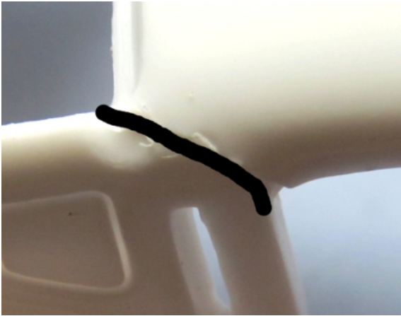
PIC 42 PIC 43 The rear roof area has strong mold lines. Remove the injection sprue from the window very carefully. Clean up the window area.
