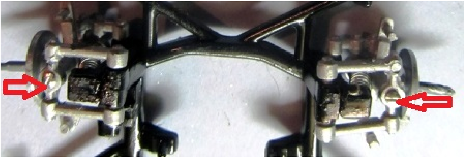
PIC 10 Use the screws and attach an upper and lower A-arm to each spindle. There is a small tab on both the lower A-arm and the upper frame mount that the spring sits on to.
