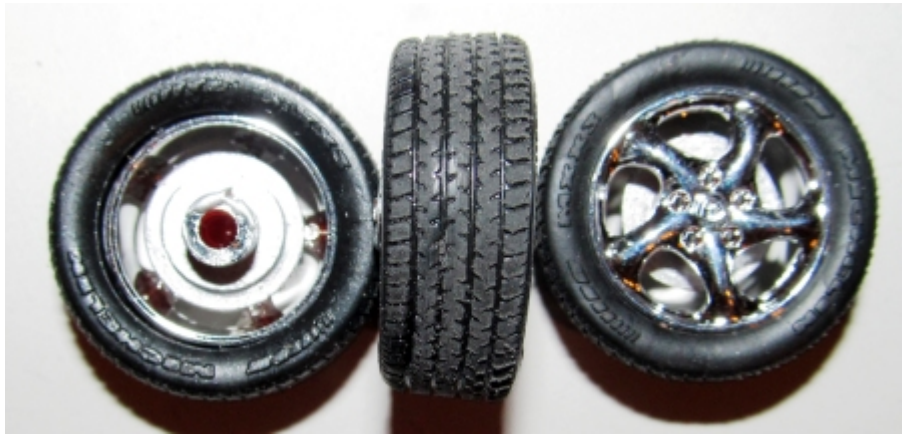
PIC 17 PIC 18 The tires are assembled next. These are Non-Directional and all the same size. There is no need to worry about location. To give the tires a road used look press the tread on a sheet of 220 grit sandpaper and roll the tread moving the tire. This will rough up the tread. Paint the brakes Silver and install onto the axle posts. Insert the rims into the tires.
