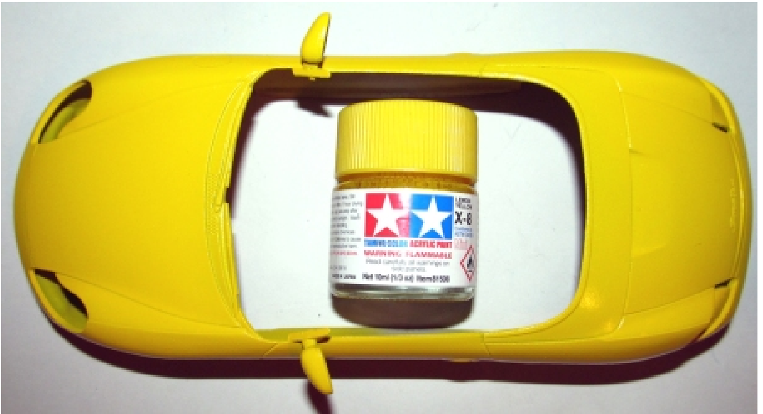
PIC 26 I used Tamiya Lemon Yellow (X-8) for the base body color on this build. Mix the bottle 60/40 with Thinner, or the consistency of Skim Milk, and spray thin even coats with the airbrush. Build the color slowly as not to cause runs.
