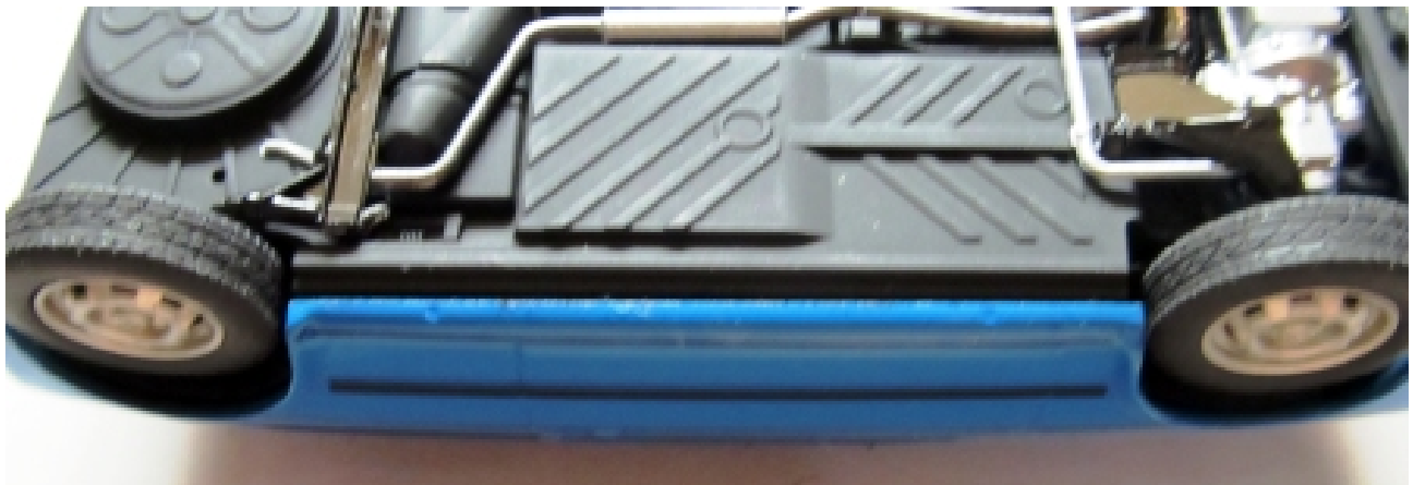
PIC 44 Shoehorn the whole unit into the body. Line up the dash, wheel wells and engine bay and it will tightly slide into place without the need for glue.
