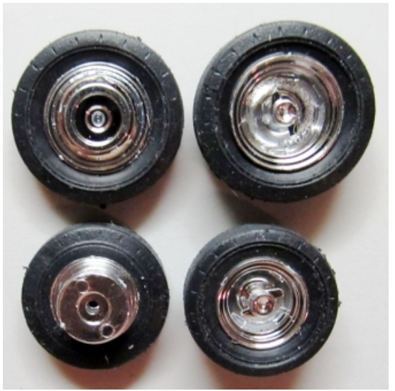
PIC 18 PIC 19 The tires need to be assembled. Take note the SMALLER tires are in the front of the car. To give the tires a road used look roll and press the tread on 220 grit sandpaper. Install the spinner onto the hub center. Insert the rim into the tire. Add the trim ring. Do all four tires this way. On the FRONT add the brake drum and inner wheel. On the REARS only add a brake drum.
