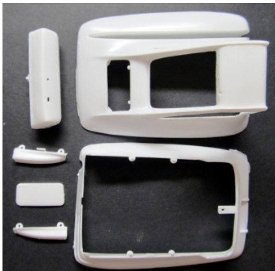
PIC 25 PIC 26 The body can be completely assembled prior to any paintwork. Trim any flash and rough edges. Glue the upper half to the lower half. Add the wheel wells and the rear panel. The hood is left loose.
