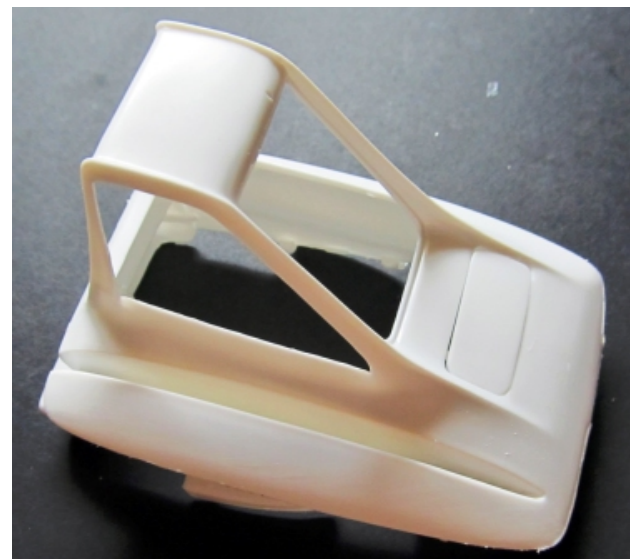
PIC 25 PIC 26 The body can be completely assembled prior to any paintwork. Trim any flash and rough edges. Glue the upper half to the lower half. Add the wheel wells and the rear panel. The hood is left loose.
