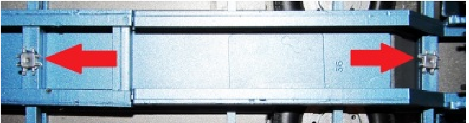
PIC 44 Paint the hydraulic transfer boxes Aluminum and install on the underside.
