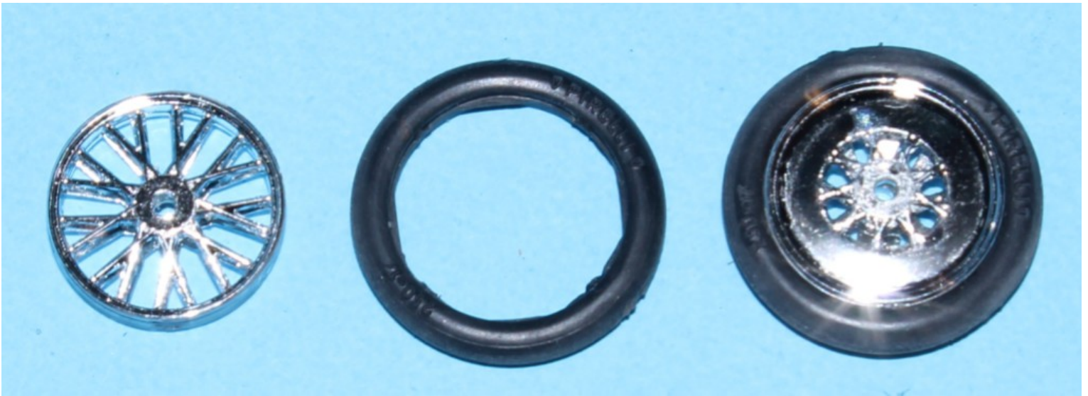
Pic 18 The rims halves were then glued together and the tire put on. The fronts were then set aside to dry thoroughly.
