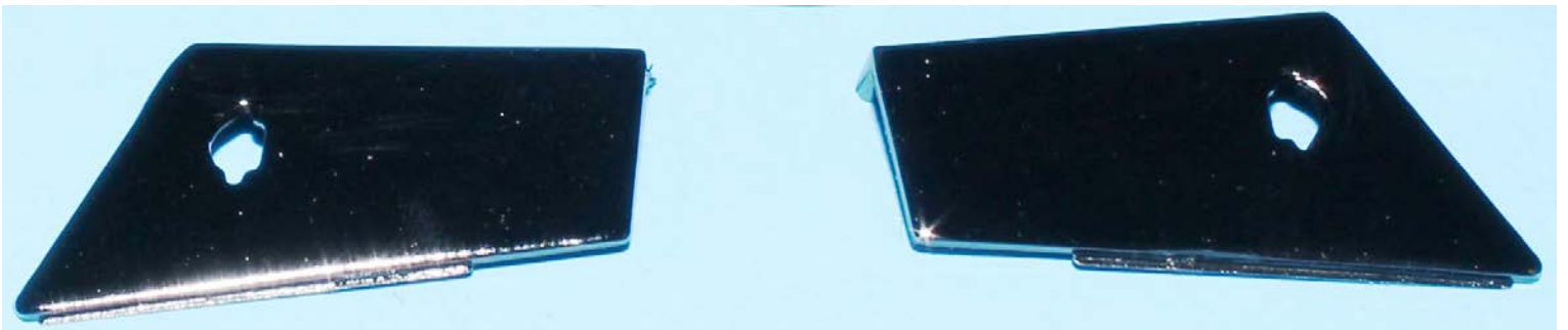
Pic 27 With everything coming together nicely and the chassis done, it was now time to start adding the body panels. The first two added are the driver's compartment side/bottom panels. These two panels, as well as the rest, had been painted DC Gloss Black Lacquer earlier, and had been clear coated using DC #DAL 1695 Acrylic Lacquer Clear, numerous times giving a high-gloss finish. These panels have the rear end axle holes in them and fit over the axles and I glued them together along the bottom joint and where they touch the frame (using just a small drop of tube glue) on the frame locations.
