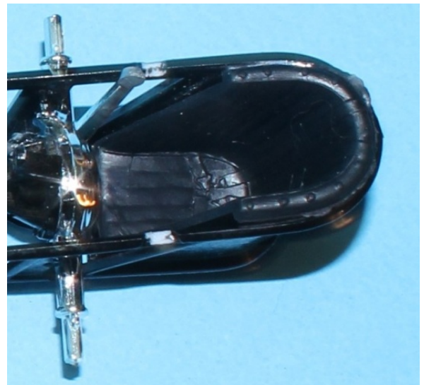
Pic 13 Pic 13a The first steps in the chassis assembly are to install the rear end and the long control. ***NOTE***: Make sure you install the rear end with gear (pumpkin) as shown in the instructions otherwise you can't get the rear end through the frame to install it. Once I had the rear end and lever in place I glued the pumpkin to the front and then the drive shaft to the mount and the pumpkin. Both the parts had been pre-painted using Model Master (MM) enamels, the pumpkin Gloss Black and the drive shaft Steel.
