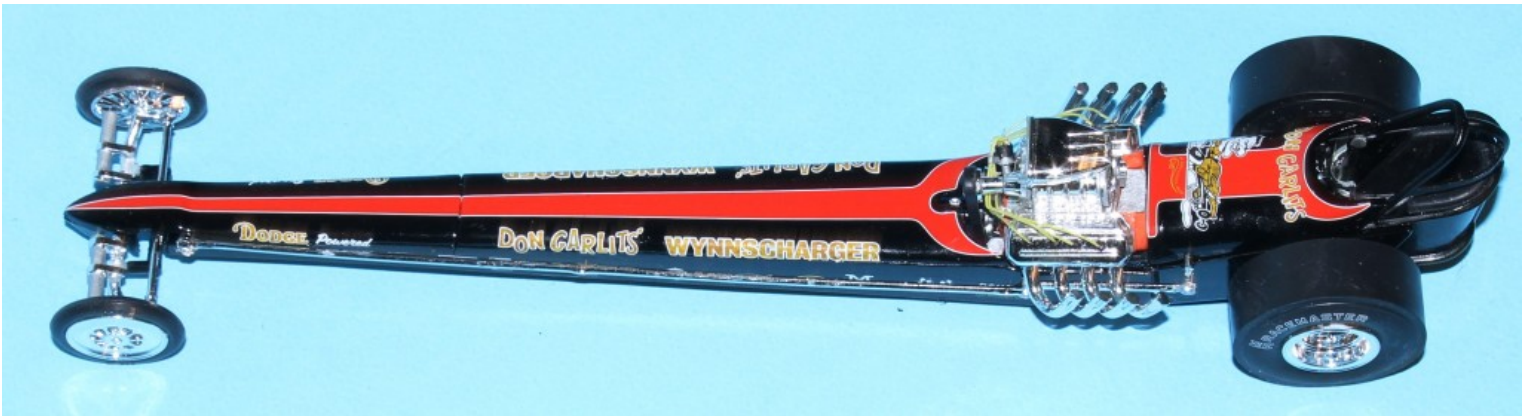
Pic 31 Before gluing the windshield and parachute in place I applied the decals using the Microscale two-part system. The instructions are very vague in the placement of the decals on the sheet and explain nothing about the others not shown in the line drawing of the final section on Body and Wheels. I applied the ones shown, which were the upper body red stripe the "Dodge Powered" "Don Garlits Wynnscharger" "Wynns" airfoil wing, and the sponsors.
