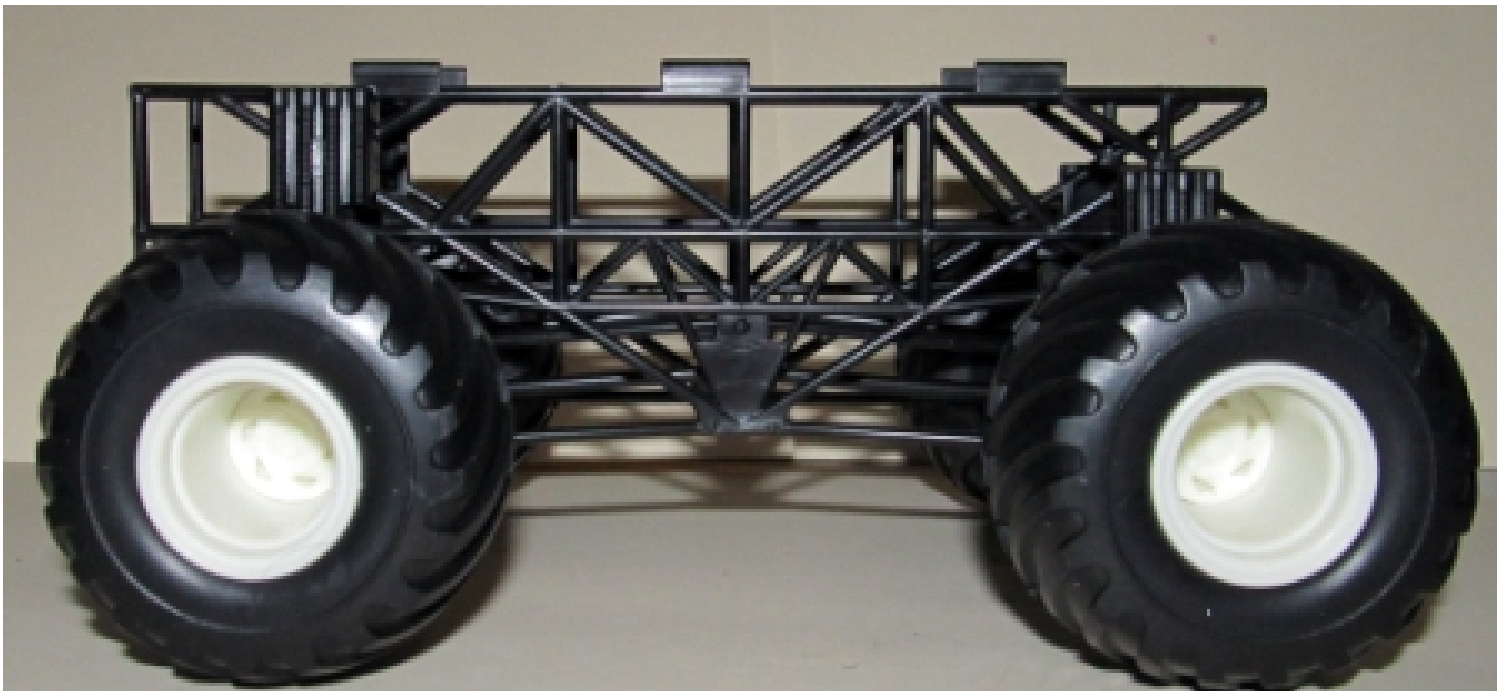
PIC 9 PIC 10 Slide an axle into each suspension and add the corresponding tire to the other side. This completes the chassis frame assembly.
