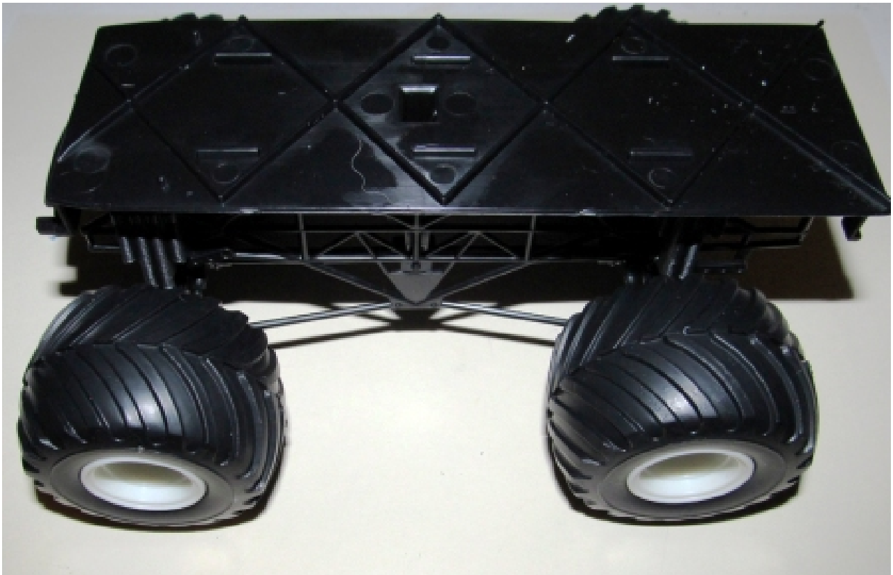
PIC 15 The instructions have you place the chassis pan into the body now. I did find that if I installed the chassis frame and wheels to the pan FIRST it made final assembly much easier. Attach the frame to the pan and then install the chassis unit into the body. This will finish the overall build.
