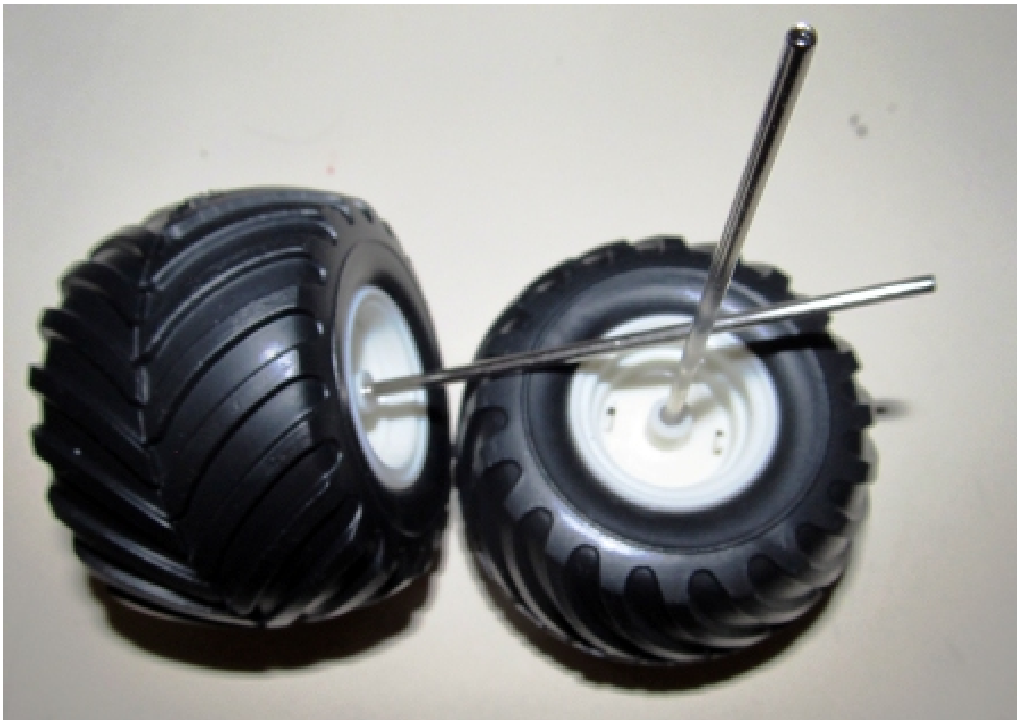
PIC 5 PIC 6 Slide the axles into the rear hole on the rims and tap lightly with a hammer to place them. Do the two matching tires so you can slide the axles into the chassis and add the opposite side. This will help ensure they are facing the proper direction.
