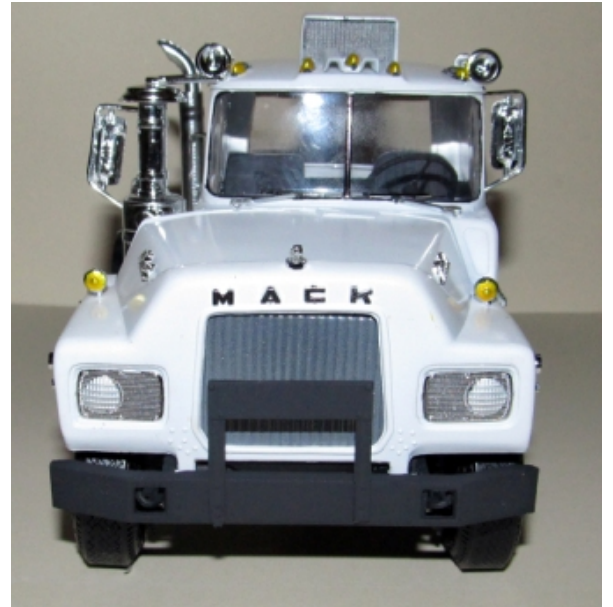
PIC 55 PIC 56 As I built a construction truck version, I used the painted bumper and push bar. Attach the bar and paint the unit Flat Black. Install that on the frame horn ends. Install the hood locks on the hood.
