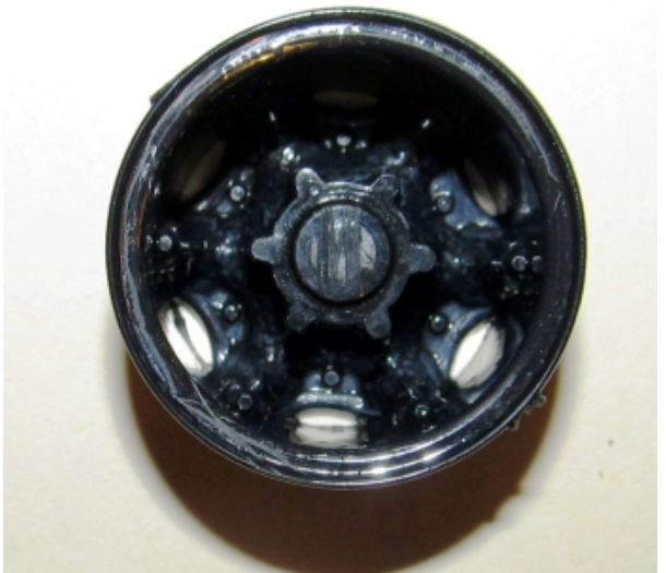
PIC 7 PIC 8 Soak the air brake parts and the outer rims in Bleach to remove the chrome. Assemble the inner rims by inserting the hub into the rear rim, glue the mid-section (deep well out), add the outer rim. Assemble and install the air brakes. Install these four units onto the axles.
