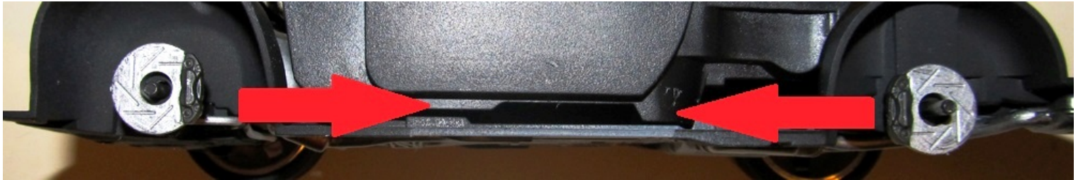
PIC 24 Install the brakes in place making sure each caliper faces IN. Insert the metal axle into the rim and install the tires smaller set in front.
