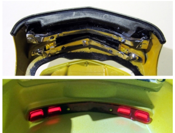
PIC 38 PIC 39 Paint the front end Satin Black. Install the headlight and fog light lenses and then the bezels into the front end. Install the front end into the body. Add the tail lights to the body. Paint the blinkers on the headlight lens Transparent Yellow.
