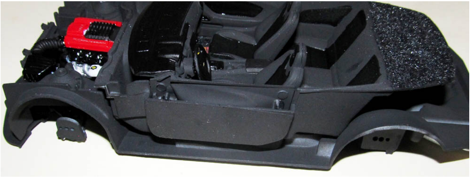
PIC 19 The interior is mounted on the chassis. Add the support bar to the shock towers and it is Black.
