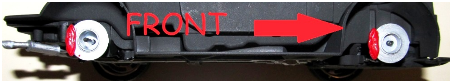
PIC 23 Install the brakes in place with the calipers to the back of the car.
