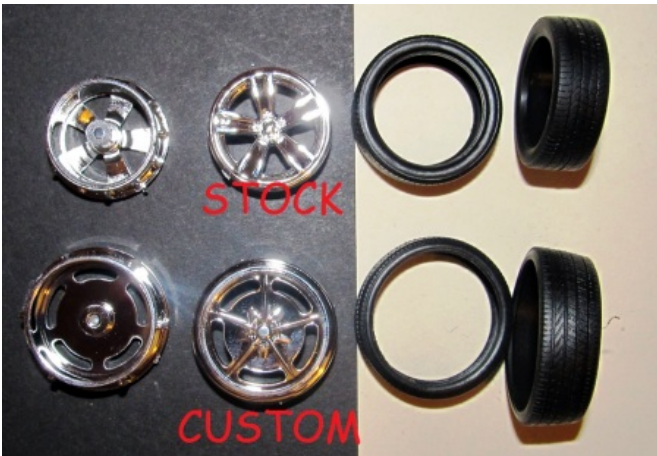
PIC 20 PIC 21 Choose between Stock or Custom wheels. Using 220 grit sandpaper press and roll the tires on the paper the rough up the surface to give the tires a worn look. Install the tires onto the rims. There is a small and large tire so make sure you put the tires on the proper rim and location.
